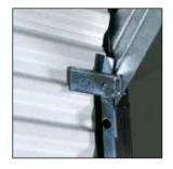
12-gauge, zinc-coated door stops are mounted to brackets for increased strength. 18-gauge, zinccoated steel guides with polypropylene runners allow doors to glide smoothly.
