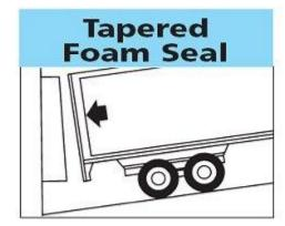
IF AN inclining or declining ramp is a problem, NOVA SEAL offers a solution. Sides of foam seal can be tapered to match the angle of the ramp.
